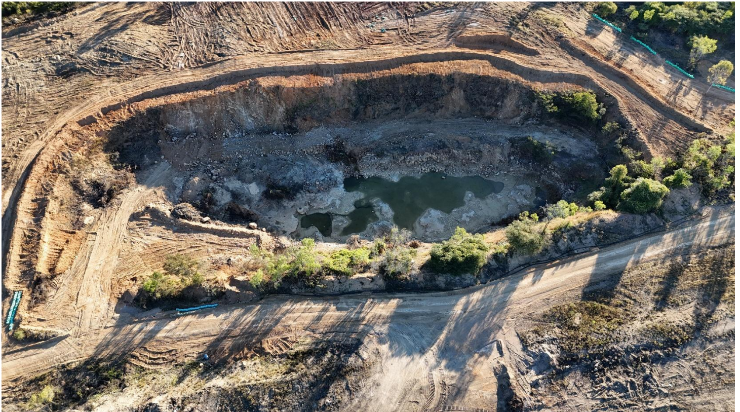
Figure 11: Initial open-pit benching development
